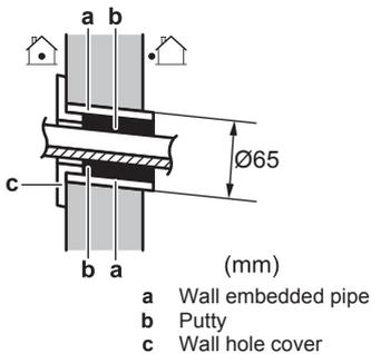
**Note:** After completing wiring, refrigerant piping and drain piping, do NOT forget to seal the gap with putty.
