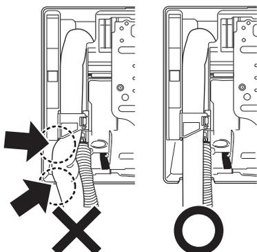
2 Pass the drain hose and refrigerant pipes through the wall hole.
