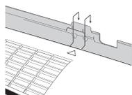
2 Press the bottom frame of the unit with both hands to set it on the bottom hooks of the mounting plate. Make sure that the wires do NOT get squeezed anywhere.
